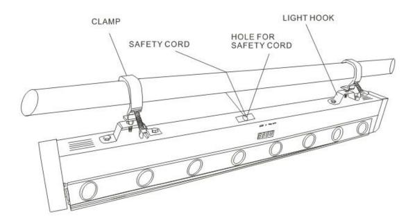
Use 2pcs clamp (need to purchase).Use clamp fix with light hook which in the packing box with light, then use fastlock install to the bottom of lamp. Hang the fixture on the structure and fasten the screw attached to each clamp. Make sure the light is installed reliable, and confirm the light which you fixed is strong enough for hanging the light. Base on safety reason, please according to the above picture using safety wire cross the light to make it strong enough again.
