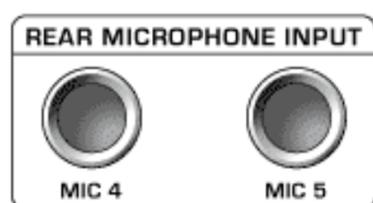
There are two microphone inputs (1/4" slot) on the rear panel.
